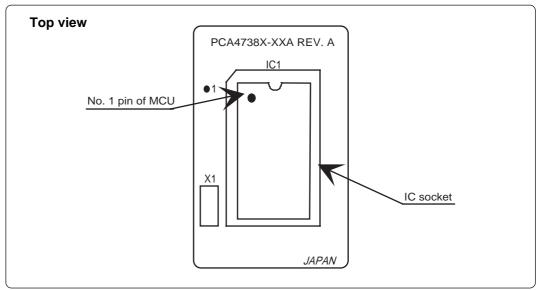
Figure 3.5 Mounting an MCU (adapters with DIP type IC socket)
